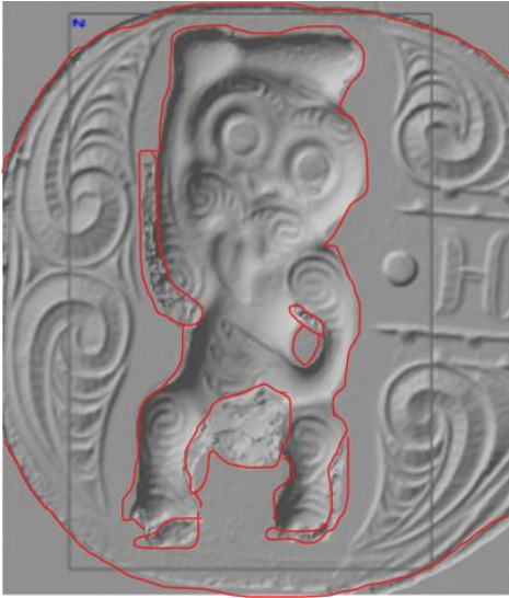
Figure 3: Errors in STL highlighted in red
