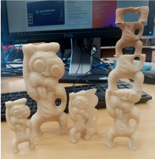
Figure 7: Some of the test prints, unfinished prints on right either due to clogging or time constraints
