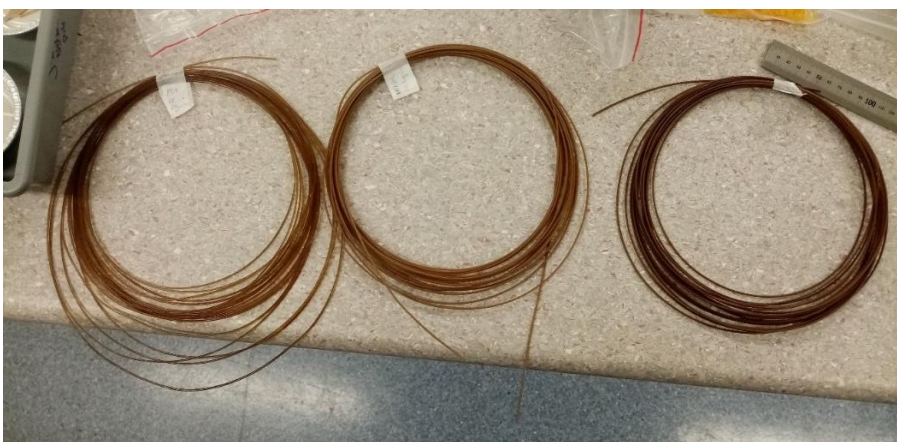
Figure 6: Filaments with 1% lignin - 0% Harakeke (left), 1% lignin – 10% Harakeke (centre) and 2% lignin – 10% Harakeke (right)
