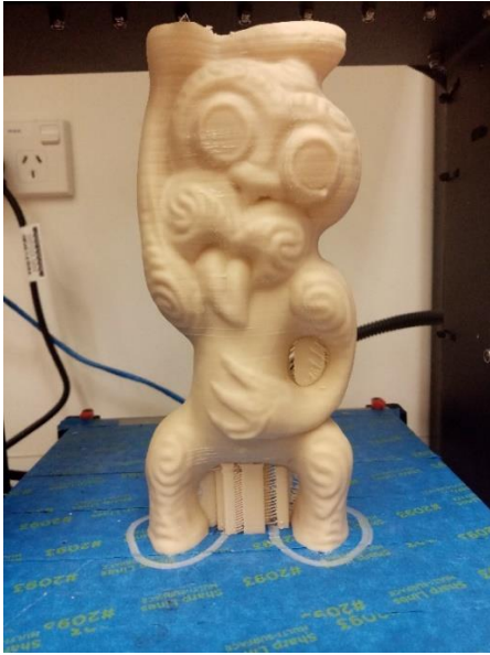
Figure 8: The final printed model, with supports and skirting
